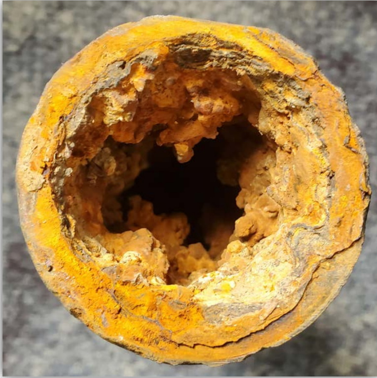
Sediment Buildup & Corrosion of Aging Waterlines (5 Year CIP includes replacing similar condition waterline on Quincy Boulevard and 4 th Street Terrace)
